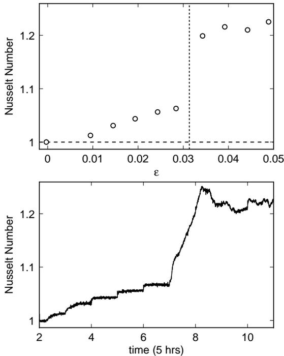
FIG. 17. Nusselt-number measurements for  $h = 61$  in cell 5. The upper figure illustrates the dependence of the Nusselt number on  $\epsilon$ . The dotted line indicates  $\epsilon_n$ , where the transition from hexagons to rolls occurred when  $\Delta T$  was increased. The lower figure illustrates the dependence of the Nusselt number on time. Time is measured in units of 5 hours, i.e. the time between steps in  $\epsilon$ .
