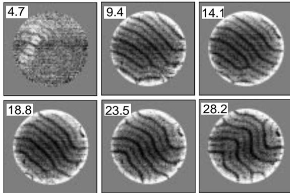
FIG. 11. A temporal succession of images during the transient leading from conduction to convection when  $\Delta T$  was raised slightly above  $\Delta T_c$  for cell 5. The field was  $h = 50$ . The numbers are the elapsed time, in units of  $t_v$ , since the threshold was exceeded.
