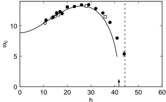
FIG. 7. The Hopf frequency  $\omega_c$  as a function of  $h$ . Open and filled circles are for cells 4 and 5, respectively. Open squares are for cell 6. The solid line is the theoretical prediction for  $\omega_c$ . The dashed line (arrow) indicates the location of the codimension-two point as found experimentally (theoretically).
