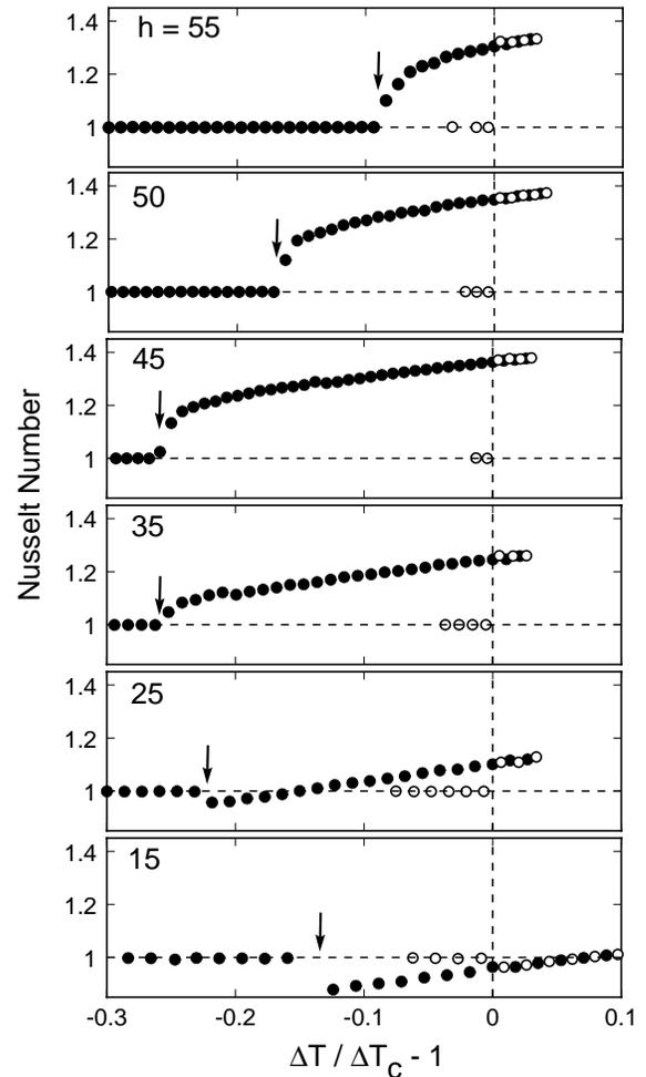
FIG. 12. Nusselt-number measurements for cell 5 illustrating the variation of the size of the hysteresis loop between conduction and convection with  $h$ . The number in the upper left corner of each plot is the field  $h$ . Open circles were taken with increasing and solid circles with decreasing  $\Delta T$ . The arrows show the values of  $\epsilon_s \equiv R_s/R_c - 1$ .
