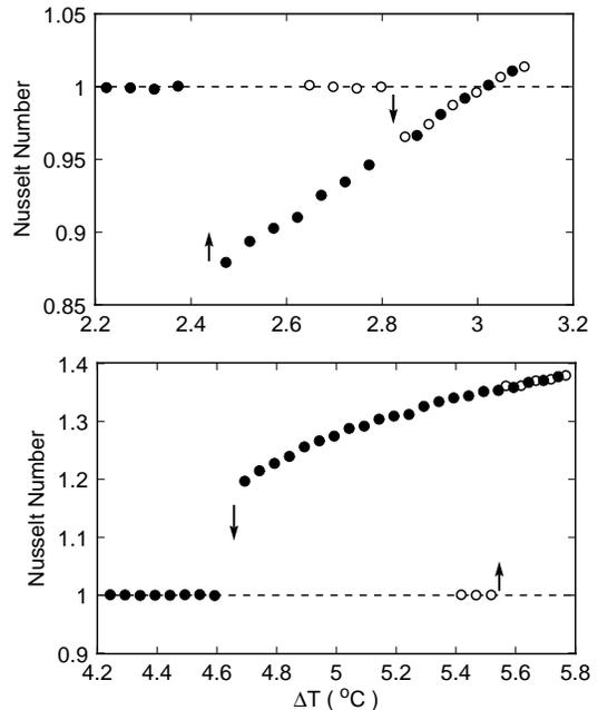
FIG. 1. Examples of the Nusselt number as a function of  $\Delta T$  for cell 5. The upper figure is for  $h = 15$  and the lower one is for  $h = 50$ . Open circles were taken with increasing and solid circles with decreasing  $\Delta T$ . The transitions between conduction and convection are indicated by the arrows.
