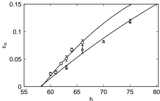
FIG. 18. Values of  $\epsilon_n(h)$  where a transition to a spatially and temporally chaotic state occurred. Circles and triangles were obtained in cells 5 and 6, respectively. The lines represent a fit of a quadratic polynomial in  $(h/h_n - 1)$  to the data. The fits extrapolate to zero at  $h_n = 58.3 \pm 0.7$  for cell 5 and  $h_n = 58 \pm 3$  for cell 6.
