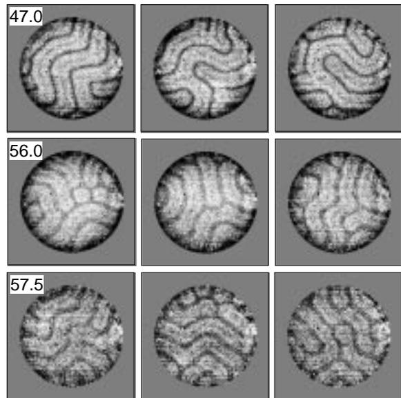
FIG. 23. Time sequences of the spatially and temporally chaotic flow for  $R = 4000$  and at different values of  $h$  for cell 5. The images in each row were taken at the field indicated in the leftmost image. Time increases from left to right. Images were taken in one hour intervals. The wavenumbers of the patterns are  $h = 47$ :  $k_n = 3.4$ ,  $h = 56$ :  $k_n = 3.6$ ,  $h = 57.5$ :  $k_n = 3.9$ .
