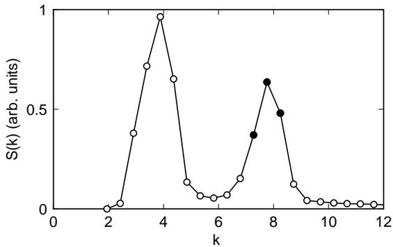
FIG. 8. The azimuthal average of the time-averaged structure factor  $\langle S(k) \rangle$  of the travelling/standing wave transients at  $h = 32$  for cell 5. The mean wavenumber calculated from the solid circles was used as the critical wavenumber.
