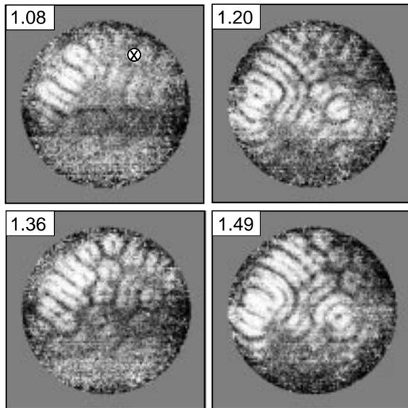
FIG. 5. A sequence of images of the travelling/standing wave transients for  $h = 32$  and  $\epsilon = 0.015$  in cell 5. The number in each image corresponds to the time, in units of  $t_v$ , that elapsed since flow first became visible. A time series of the pixel intensity was taken at the location marked in the top left image.
