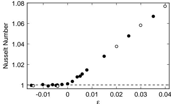
FIG. 14. Nusselt-number measurements for  $h = 63$  and cell 5 illustrating the supercritical nature of the bifurcation characteristic of the high fields. Open circles were taken with increasing and solid circles with decreasing  $\Delta T$ .
