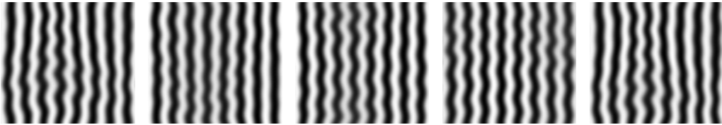
FIGURE 18. Complex travelling wave pattern for \gamma = 0.5^\circ , \epsilon = 0.172 , \epsilon_0 = 0.163 , L_x = 8\lambda_c(\gamma) , L_y = 0.906L_x . The pictures are sorted increasing in time from left to right at t = 3728, 3741, 3779, 3804, 3851t_v . For the travelling waves we find \omega = 1.62 .
