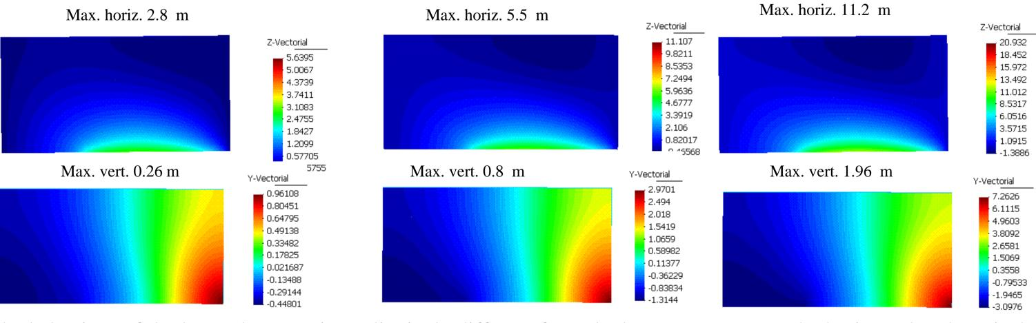
The behaviour of the layered system is qualitatively different from the homogenous one. The horizontal and vertical deformation patterns are unsymmetric. The maximum horizontal and vertical deformations depends strongly on the shear moduli ratio.
