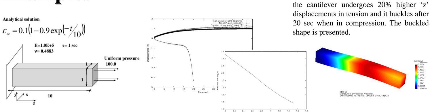
A simple geometrical model of a cantilever (fixed at z=0 in z direction), with a known linear visco-elastic analytical solution, is compared against the FEM model that is discretized with 13824 tetrahedra (10 nodes). The fine discretization is undertaken to evaluate the speed-up effect when solved in parallel. The scaling effect is shown above as well.
