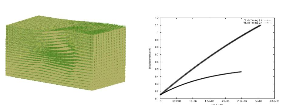
This figure presents dependence of the vertical deformation of a point on the surface on time for two different ratios of the shear moduli (Emu). The higher ratio gives results closer to the Maxwell model characteristics
