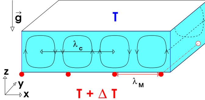
Figure 1. A sketch of a thermal convection cell. Beyond a critical temperature difference  $\Delta T$  between the lower and the upper container boundary convection rolls bifurcate from the heat conducting state. The temperature difference may be also spatially periodic modulated with a modulation wavelength  $\lambda_m$ , as indicated by the read heat wires.
