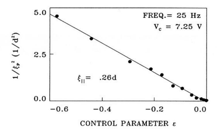
Figure 3: The correlation length as measured parallel to the director orientation at a driving frequency of 25 Hz. The slope of the fitted straight line yields the value of  $\xi_{\parallel} = 0.26d$ .
