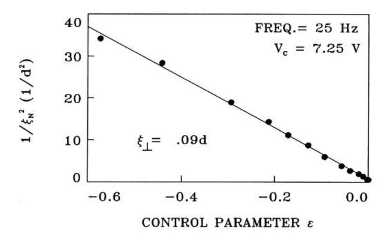
Figure 4: The correlation length as measured perpendicular to the director orientation at a driving frequency of 25 Hz. The slope of the fitted straight line yields the value of  $\xi_{\perp} = 0.09d$ .
