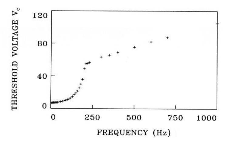
Figure 1: The phase diagram. The crosses indicate the critical voltage for the onset of convection.
