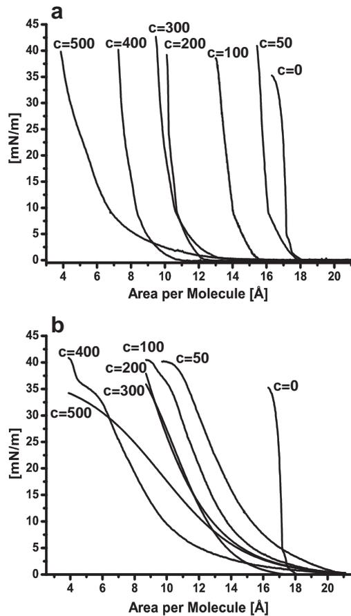
Fig. 2. Surface pressure ( $\pi$ ) – area (A) isotherms of MO monolayer at temperature  $T = 22$  °C at different subphase surfactant concentrations for (a) SDS and (b) DTAB.
