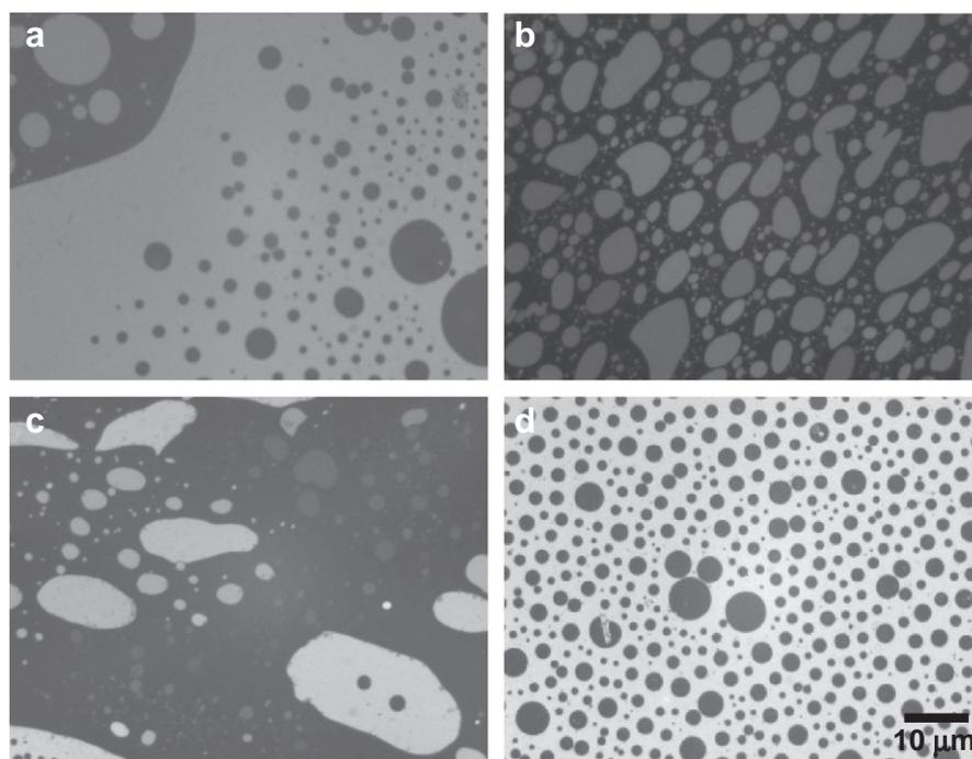
**Fig. 4.** Fluorescence microscopy images of MO monolayer at  $\pi = 5$  mN/m and  $T = 22$  °C on a pure water (a) and 200  $\mu$ M SDS (b). Images (c) and (d) are the same as (a) and (b) but at pressure  $\pi = 10$  mN/m.
