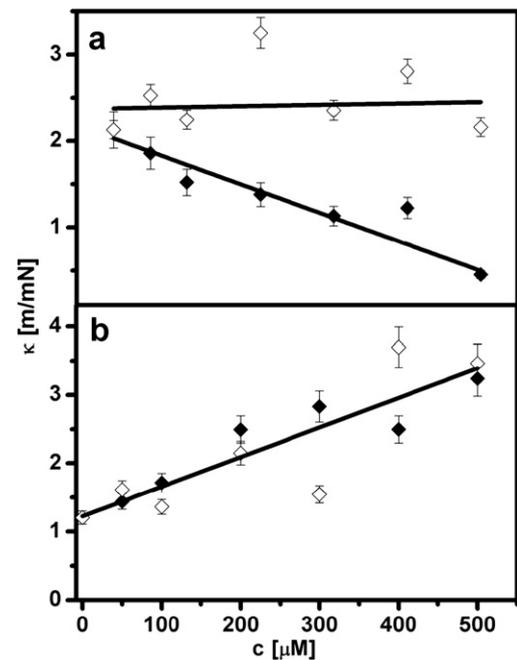
Fig. 3. Variation of surface compressibility modulus of MO monolayer at constant temperature as a function of subphase surfactant concentrations at pressure (a)  $\pi = 5$  mN/m, and (b)  $\pi = 10$  mN/m. The symbols in the figure are ◆ for SDS and ◇ for DTAB.
