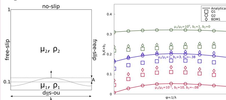
Figure 4: Benchmark setup for Rayleigh-Taylor instability. The jump in density and viscosity is following a small perturbation of amplitude  $A$  at  $z = 0.1$ . For different viscosity contrasts and wavelengths  $\lambda$  the growth factor  $K$  has been computed.  $b_1, b_2$  have been chosen such that the plots fit into one figure.
