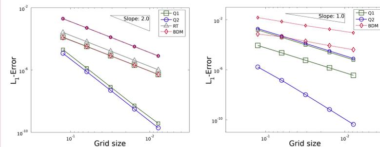
Figure 3:  $L_1$  errors of the four elements for velocity (large markers) and pressure (small markers) for the isoviscous setup (left,  $\mu_1 = \mu_2 = 1$ ) and the variable viscosity setup (right,  $\mu_1 = 1$ ,  $\mu_2 = 10^3$ ).
