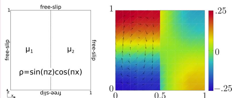
Figure 2: Benchmark setup with lateral viscosity jump. Analytical velocity (arrows) and pressure (colorbar) solution for  $\mu_1 = 1$ ,  $\mu_2 = 10^3$ .
